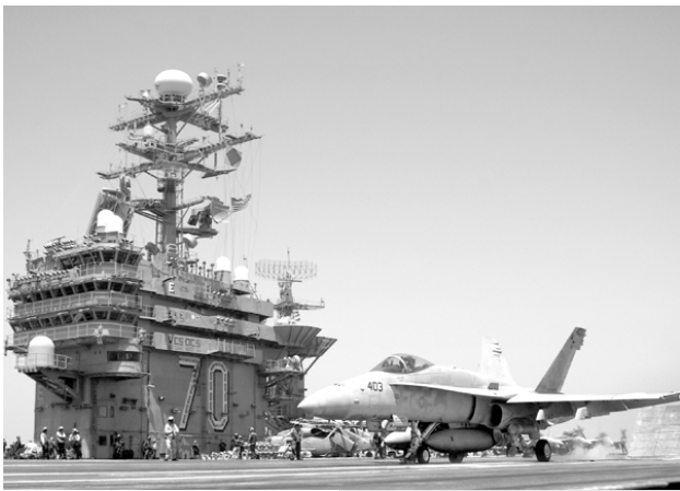
— U.S. Navy Photo by Photographer's Mate 2nd Class Inez Lawson An F/A-18C Hornet from the “Argonauts” of Strike Fighter Squadron One Four Seven (VFA-147) launches from one of four steam-powered catapults on the flight deck aboard the Nimitz-class aircraft carrier USS Carl Vinson (CVN 70). The Carl Vinson Carrier Strike Group is currently deployed to the Persian Gulf conducting operations in support of multinational forces in Iraq. Vinson will end its deployment with a homeport shift to Norfolk, Va., and commence a three-year refuel and complex overhaul.
