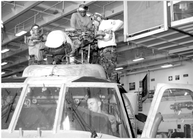
— U.S. Navy photo by Photographer's Mate Airman Recruit Ralph Zamora Sailors from Helicopter Antisubmarine Squadron One Four (HS-14) conducts a rotor head inspection on an SH-60F Seahawk in the hangar bay aboard USS Kitty Hawk (CV 63). Routine maintenance is conducted to ensure optimum levels of mission readiness and flight safety. Kitty Hawk is currently operating in the Coral Sea off the coast of Australia's Queensland region as part of Exercise Talisman Sabre 2005.
