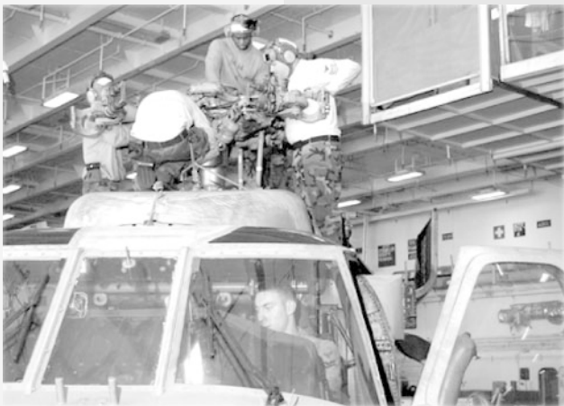
— Navy photo by Photographer's Mate Airman Recruit Ralph Zamora Sailors from Helicopter Antisubmarine Squadron One Four (HS-14) conducts a rotor head inspection on an SH-60F Seahawk in the hangar bay aboard USS Kitty Hawk (CV 63). Routine maintenance is conducted to ensure optimum levels of mission readiness and flight safety.
