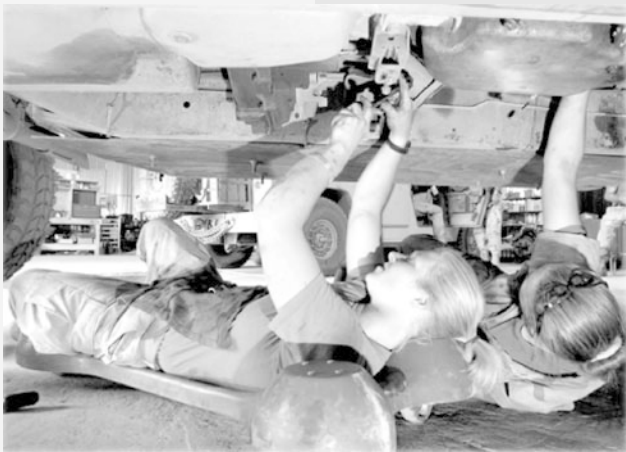
— Photo by Tech. Sgt. Christopher Gish Specs. Monica Phillips and Shiloe Weston, from the 116th Brigade Combat Team, 42nd Infantry Division, prepare to remove the transmission from a Humvee at Kirkuk Air Base, Iraq.
