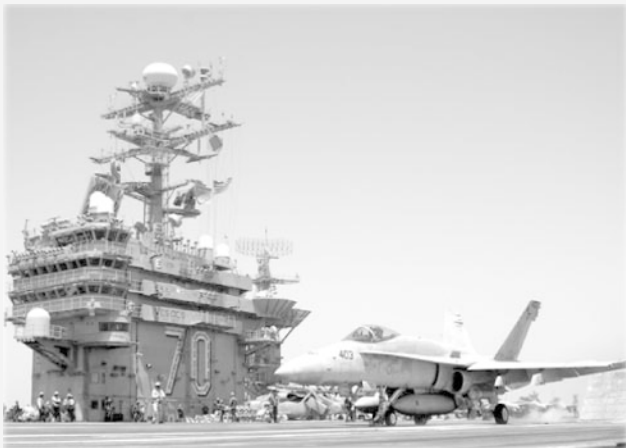
— U.S.Navy Photo by Photographer's Mate 2nd Class Inez Lawson An F/A-18C Hornet from the “Argonauts” of Strike Fighter Squadron One Four Seven (VFA-147) launches from one of four steam-powered catapults on the flight deck aboard the Nimitz-class aircraft carrier USS Carl Vinson (CVN 70).
