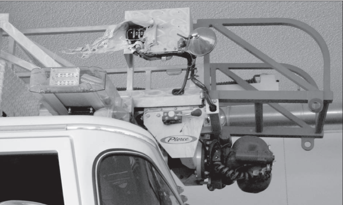
BURNT BOX – QUINT #1’s ladder control box looks like a piece of frozen flag after melting. The water cannon on the ladder is also damaged.
